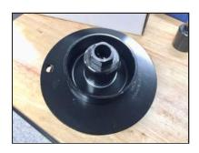
**STEP 12:** Install OEM isolator on Lift Machine. Make sure to place nub into the hole on Top Plate.
