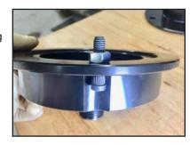
STEP 9: Important! Install white Nylon Bearing on Inner Adjustment Screw.
