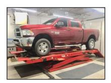
**STEP 2:** On a flat, level surface, MEASURE preinstallation ride height, FRONT & REAR, and write down measurements. Front (L)
