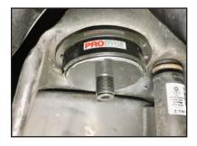
**STEP 16:** With spring still compressed, install the spring. Depending on model, it may be necessary to rotate isolator towards back of vehicle. Loosen and remove spring compressors.
