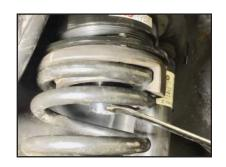
**STEP 21:** With Jam nut slightly loosened, insert 1/2" Drive extension and ratchet. Turn Inner Adjustment Screw counter-clockwise (LEFT) with ratchet to desired height. **NOTE:** Actual height of kit will be actual height of lift.
