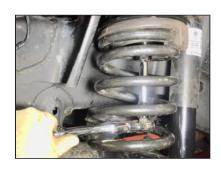
**STEP 22:** Once final height adjustment is reached, tighten Jam Nut with 1" wrench.
