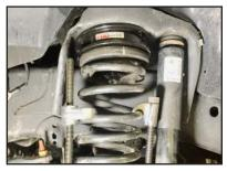
**STEP 17:** Install shock extensions using supplied hardware. Torque to **90** ft/lbs.
