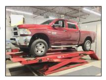
**STEP 25:** Lower the vehicle, jounce suspension and measure ride height of EACH SIDE of the vehicle, front & rear. Measure from the bottom of the wheel/rim to the lip of the fender.
